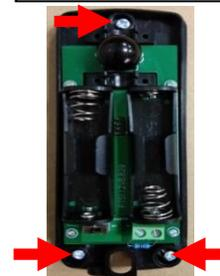
5. Put the batteries on and make the switch to Power On
